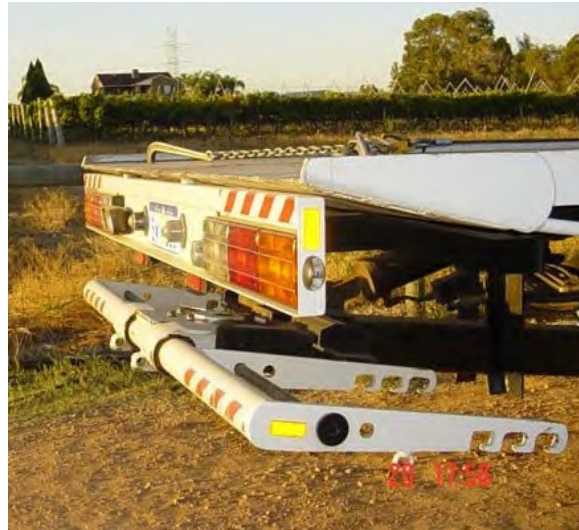
Light bar in normal position
